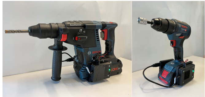
Fig. 1: Sensor system placed on hammer drill (left) and drill (right)
