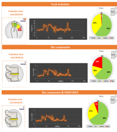
Figure 1: On-site testing, commissioning. Top: trunk inclination; middle: disc compression NoExo; bottom: disc compression wearing Paexo Back
