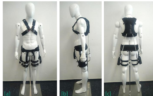
Figure 1: Complete exoskeleton with bending concept "rod modules" in front view [a], side view [b] and rear view [c].
